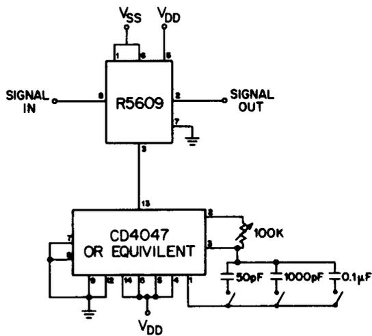
Figure 4. 100 dB/octave variable frequency low-pass filter.
