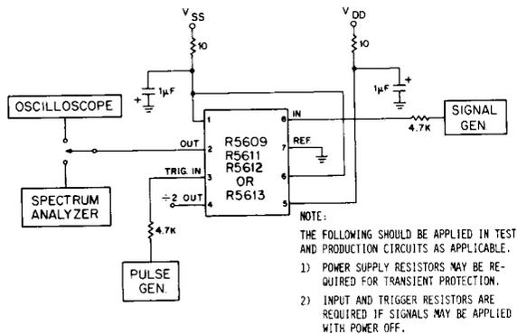
Figure 2. Test circuit for switched-capacitor filters.
