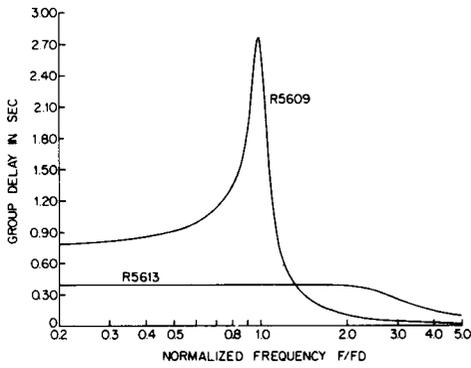
Figure 6. Group delay of R5609 and R5613 switched-capacitor filter.
