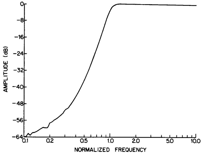
Figure 9. Frequency response of R5611 high-pass filter.
