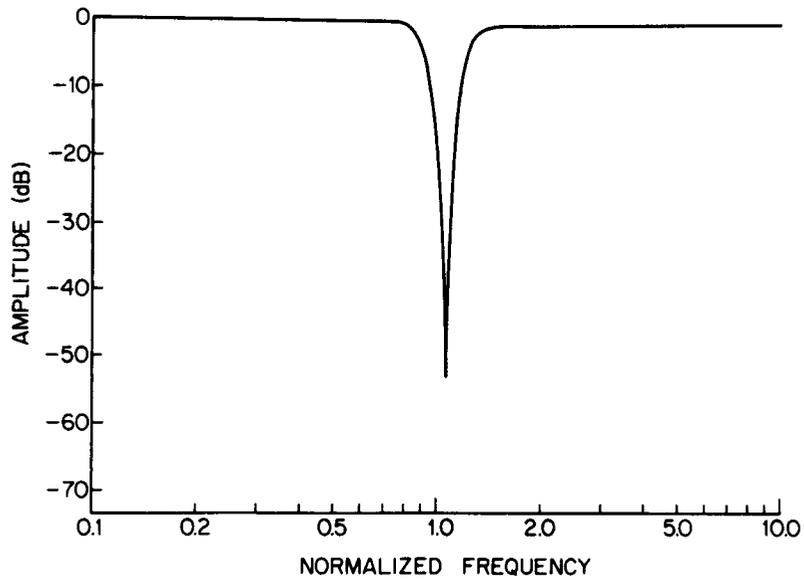
Figure 10. Frequency response of R5612 notch filter.
