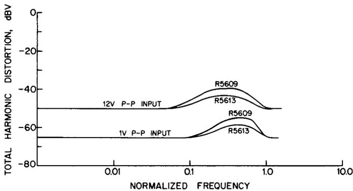
Figure 8. Total harmonic distortion. (R5609, R5613)
