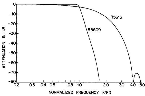
Figure 5. Magnitude response of R5609 and R5613 switched-capacitor filter.
