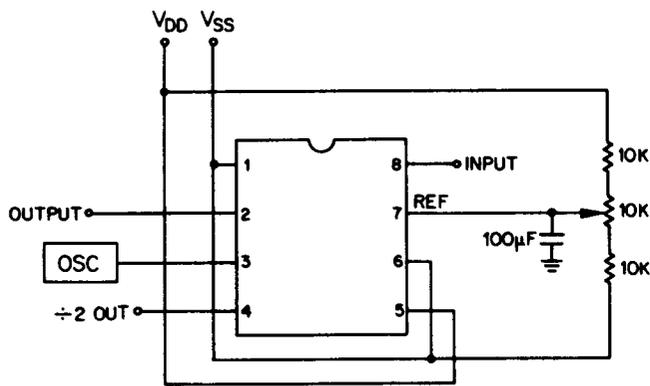
Figure 3. Circuit for nulling out the output DC offset.
